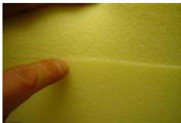
Foam layers glued correctly.
